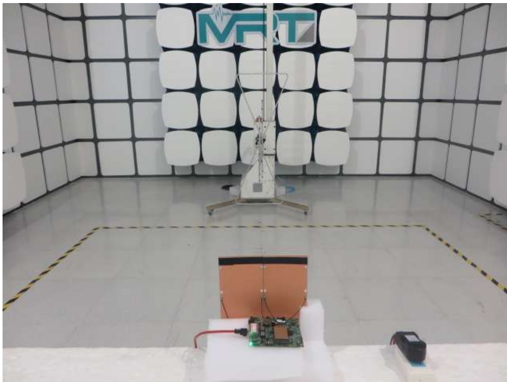
Description: Radiated Emission Test Setup for 30MHz ~ 1GHz for Panel Antenna 1#
